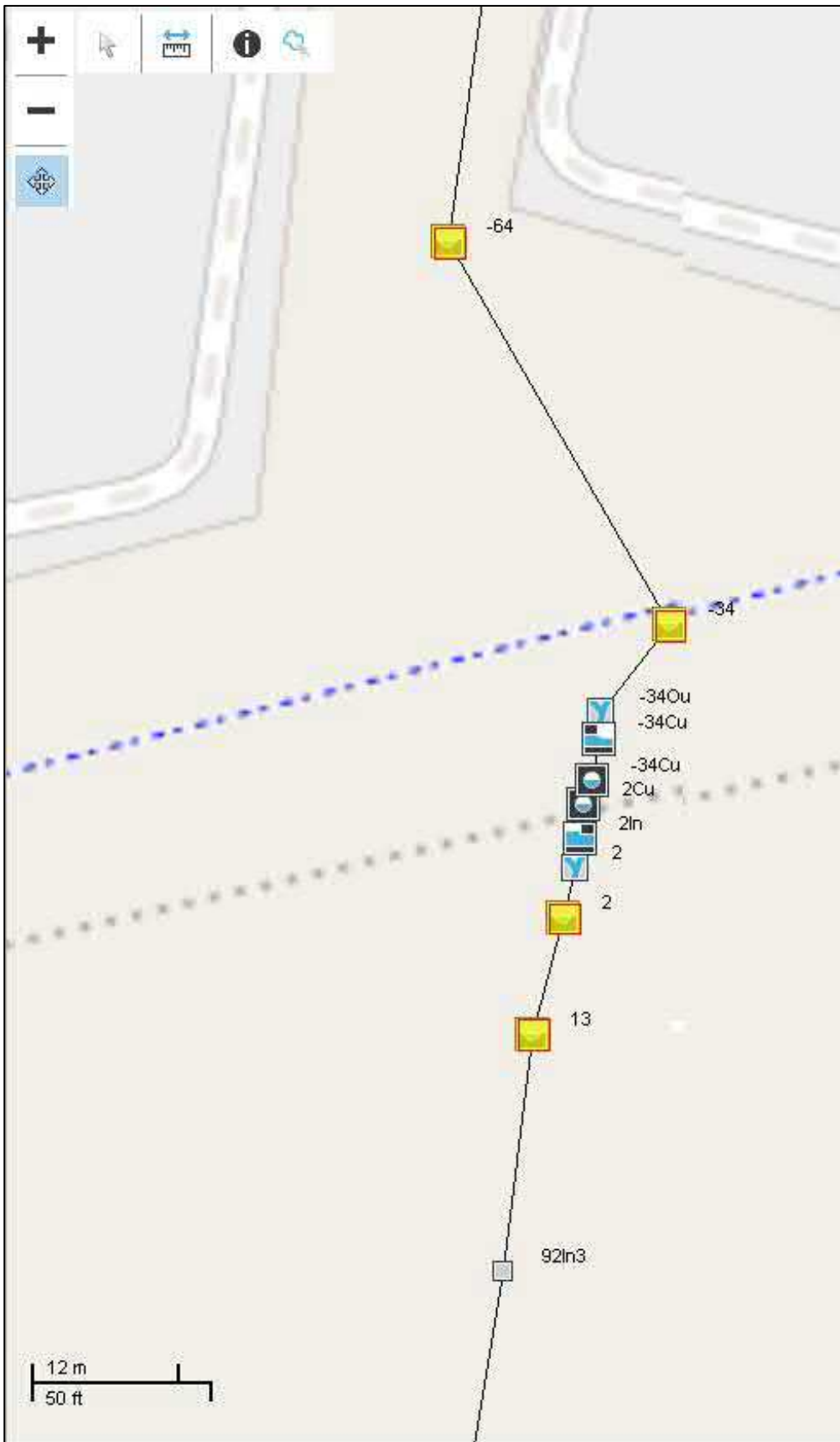
Figure 2: Peak water levels locations in 1D model domain (the grey and blue dashed lines shown are the railway and adjacent cycle path respectively)
